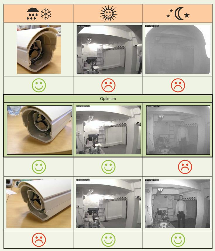
Based on results of our testing we strongly recommend using the external IR illumination for all outdoor installations where IR illumination is required.
